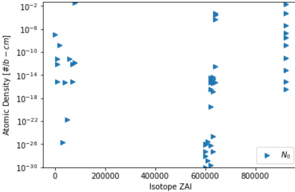
We can see that there is not a lot of change in the isotopic concentration in this depletion step. Furthermore, the classical fission yield distributions are not present due to the lack of fission yield data. Using a more complete, and typical data set, one can view the distribution of fission products more clearly, demonstrated in the below plot.
