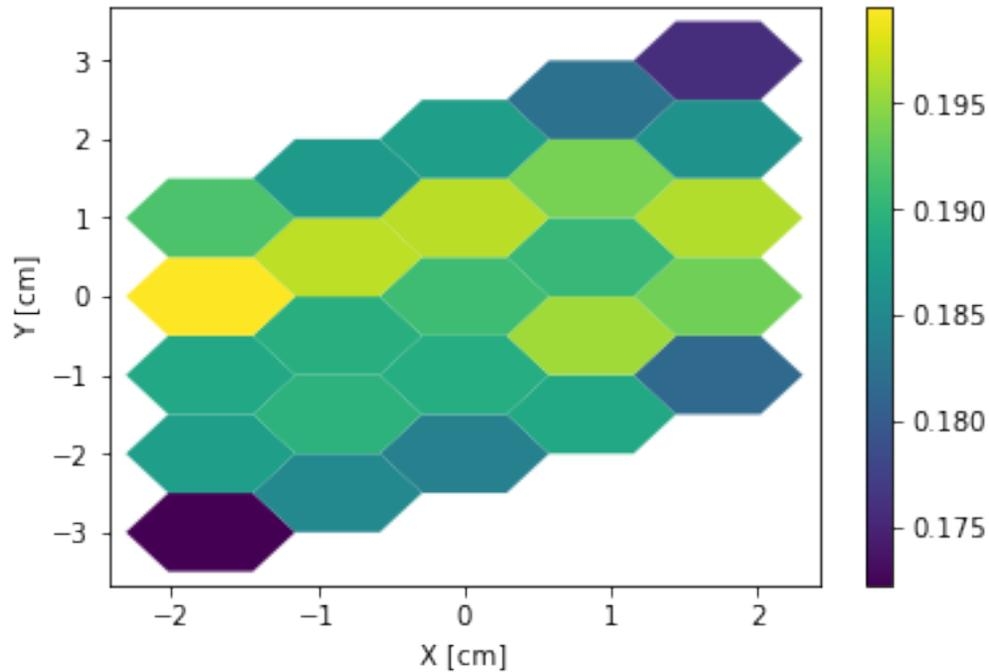
The `thresh` argument can be used to create meshes only above a given value. This works for both Cartesian meshes and hexagonal meshes.
